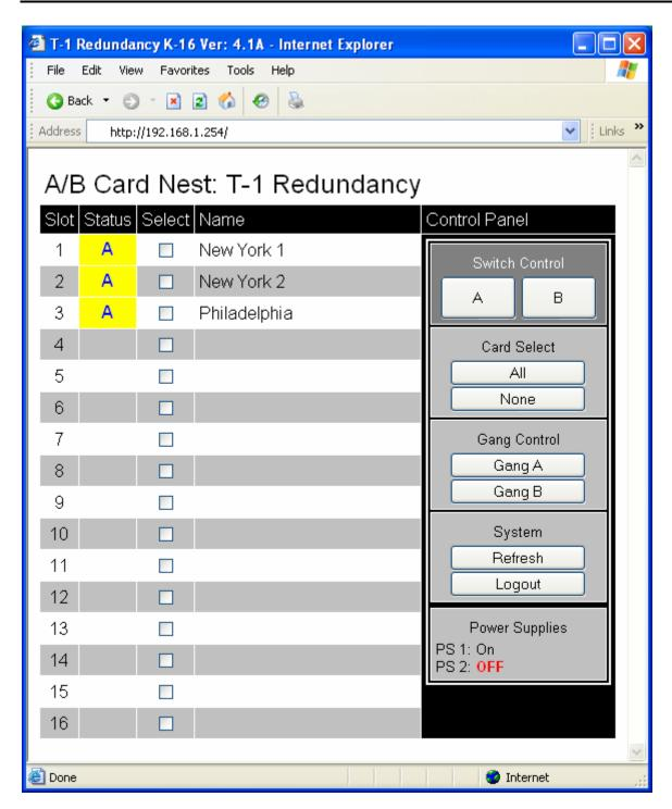
The web page shows the current status of each enabled card in the chassis. It also displays the status of the two power supplies in the lower right corner.
